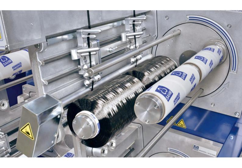
The automatic precision cross winder **CarbonStar 2-cop** maximizes efficiency by producing two bobbins (each up to 20 kg) on one winding head. Requiring only a minimum amount of space, the winder has very low maintenance costs and features metered yarn length with zero production waste – plus no downtime during bobbin changeovers.
