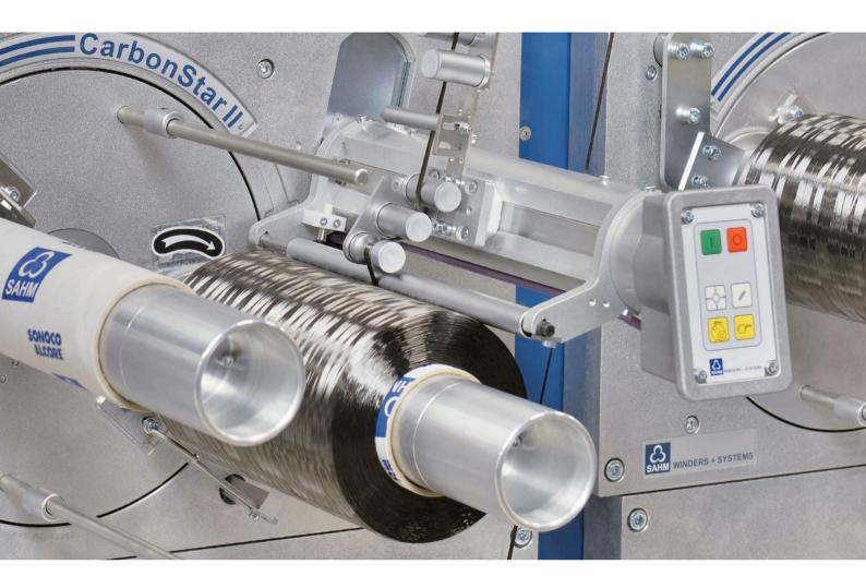
The automatic precision cross winder **CarbonStar II** requires a minimum amount of space and features metered yarn length with zero production waste – plus no downtime during bobbin changeovers.
