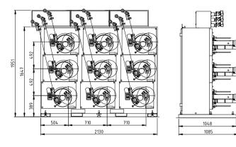
FRAME UNIT (standard with 9 winding heads - p or q wind possible)
